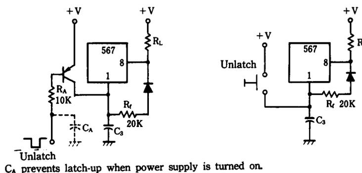
$C_A$  prevents latch-up when power supply is turned on.
