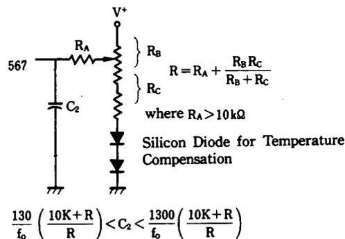
(note) Adjust control for symmetry of detection band edges about  $f_0$ .
