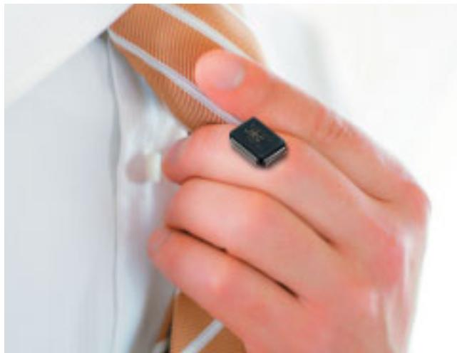
The NJW1321 is a wide band video switch with I<sup>2</sup>C Bus. It is 4-input 2-output switch with 6 dB amplifier.
