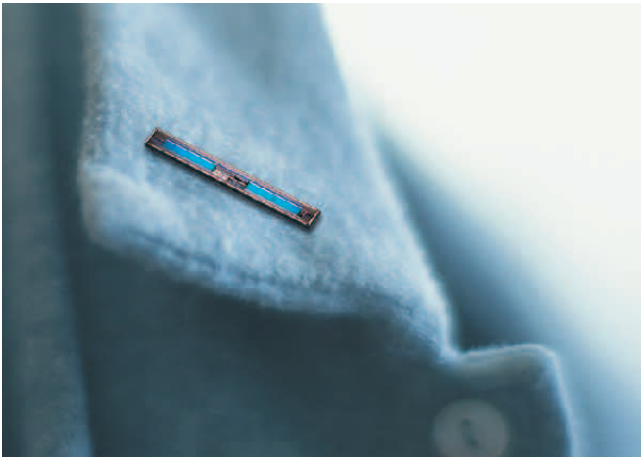
The NJU6855 is a 160COMMON × 128RGB LCD driver for 65,536-color STN display. It is suitable for battery-powered handheld applications.
